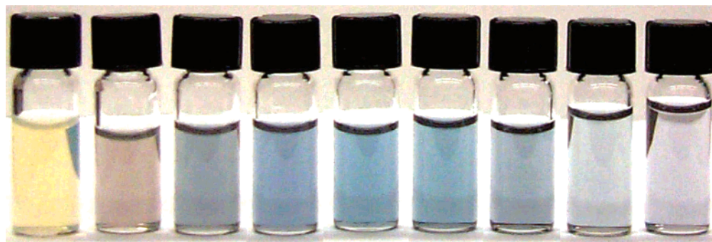
Figure 10. Photographs of aqueous dispersions of silver nanoparticles with spherical shape (see Figure 9A for a TEM image) before and after they had reacted with different volumes of 1 mM \text{HAuCl}_4 solution (from left to right): 0, 0.15, 0.25, 0.4, 0.6, 0.8, 1.0, 1.15, and 1.2 mL. Their major extinction peaks were located at 425, 451, 665, 705, 751, 793, 885, 990, and 1030 nm, respectively.
